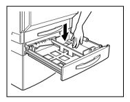
3 Remove the trailing-edge guide, and then re-install it for the size of paper to be loaded.
